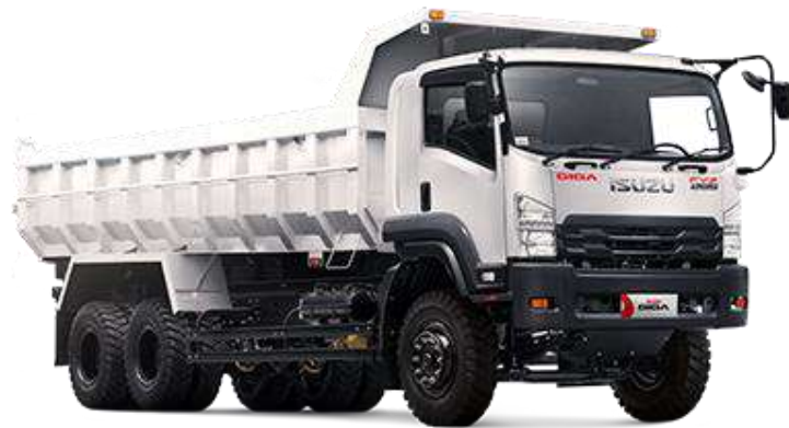
Gambar 3.11 : Dump Truck Isuzu Giga VFZ 285 PS
