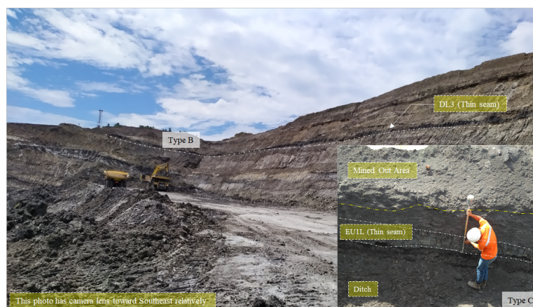
Figure 5. Field photograph of DL3 (type b) and EU1L (type c) seams.
