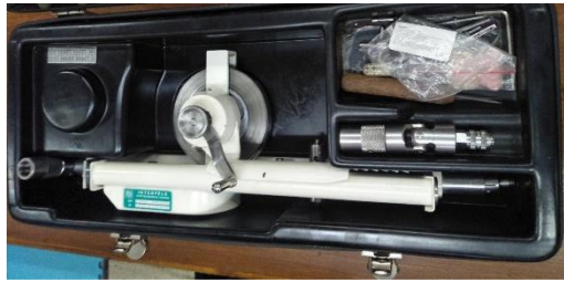
Gambar 3. Digital tape extensometer buatan Interfels
